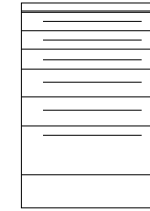
ML6 Instrument Unit (6 x Drawers) 3 x shallow drawers 2 x standard drawers 1 x deep drawer 400 / 500mm wide
