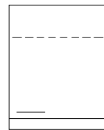
ML42 Towel / Cup Dispenser Wall Unit Dispensers Supplied By Others 500mm wide
